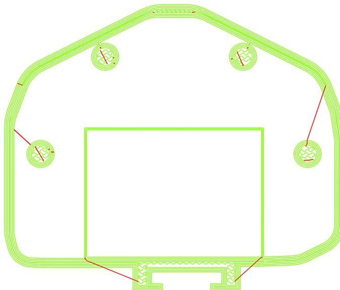
FIGURE 12. A layer of a 3D extrusion printing optimised with a TSP model. The total length of unproductive jumps for this layer is about 84.5 mm.
