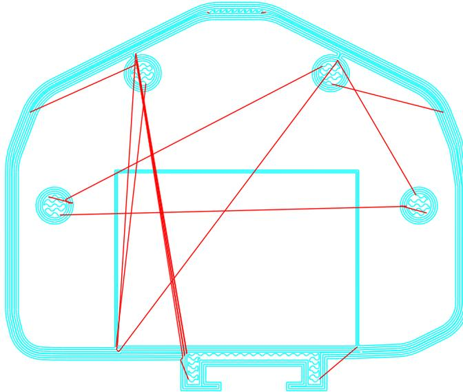
FIGURE 11. A layer of a 3D extrusion printing generated by *PrusaSlicer*. The darker segments are the unproductive jumps. The total length of these jumps for this layer is about 740.8 mm.
