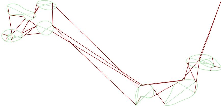
FIGURE 13. Solution found for instance 4 of Volpato et al. with head cleaning every two layers. Darker lines identify non-productive moves.
