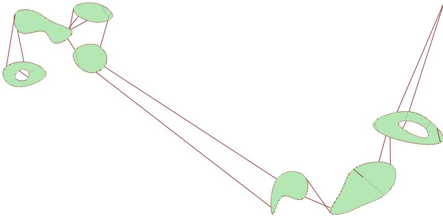
FIGURE 14. Solution found for raster filling of instance 4 of Volpato et al. Head cleaning every two layers. Darker lines identify non-productive moves.
